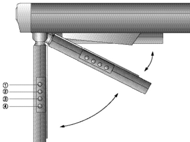
**1 MENU Button** - When pressed, the LCD control MENU is displayed.
