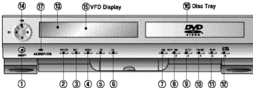
1. **ON/OFF** : Power ON /OFF and Standby Condition (Time Display).
