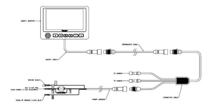
Install the **AOM713** monitor panel and wiring harness in place of the old system. Your camera cable will connect into the **TO CAMERA** inputs.
